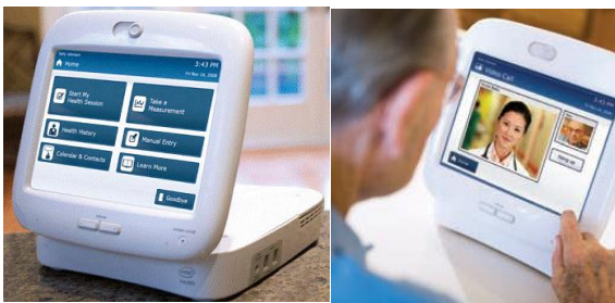
Figure 9. The Intel Health Guide Product PHS6000 showing an interactive session with a clinician in progress.
